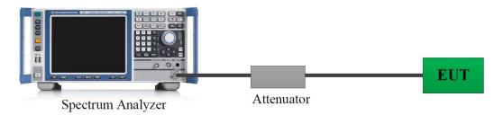
A short RF cable with low cable loss connected to the EUT antenna port, which was provided by manufacturer. The cable loss of this RF cable was offset into the setting of test equipment, which was provided by manufacturer  $\blacktriangle$ .
