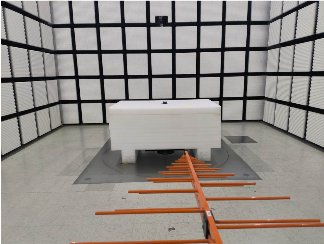
Radiated Emission Above 1GHz View
