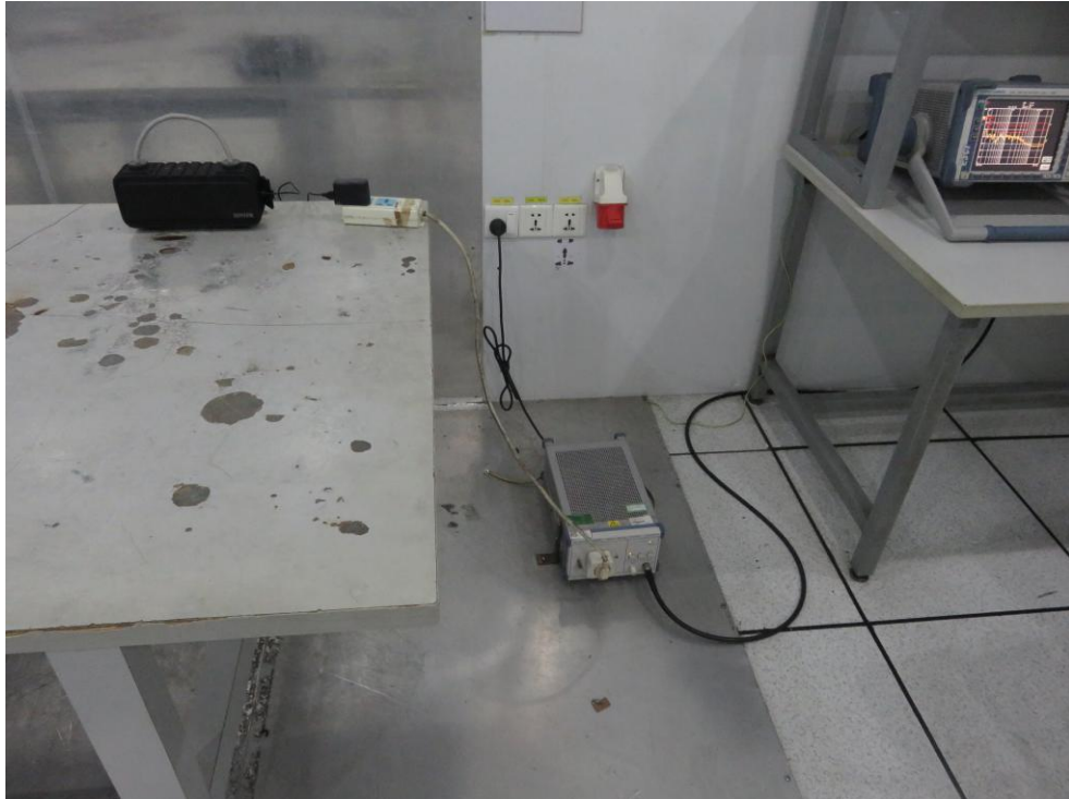
Photo of Conducted Emission Measurement
