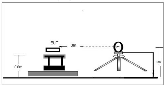
(B) Radiated Emission Test-Up Frequency 30MHz~1GHz
