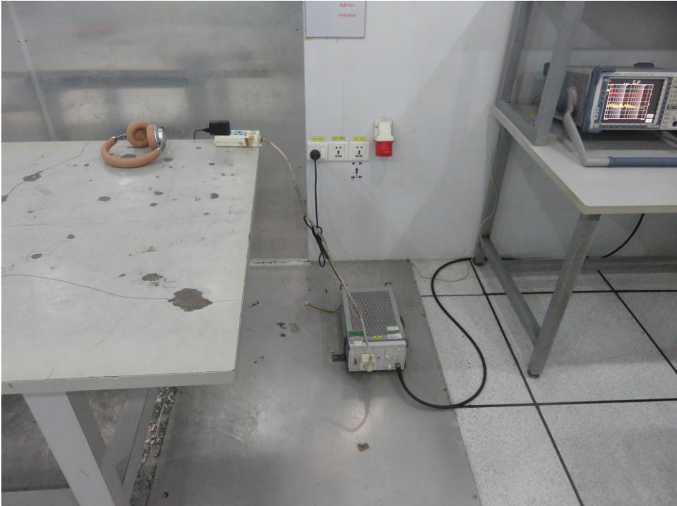
Photo of Conducted Emission Measurement
