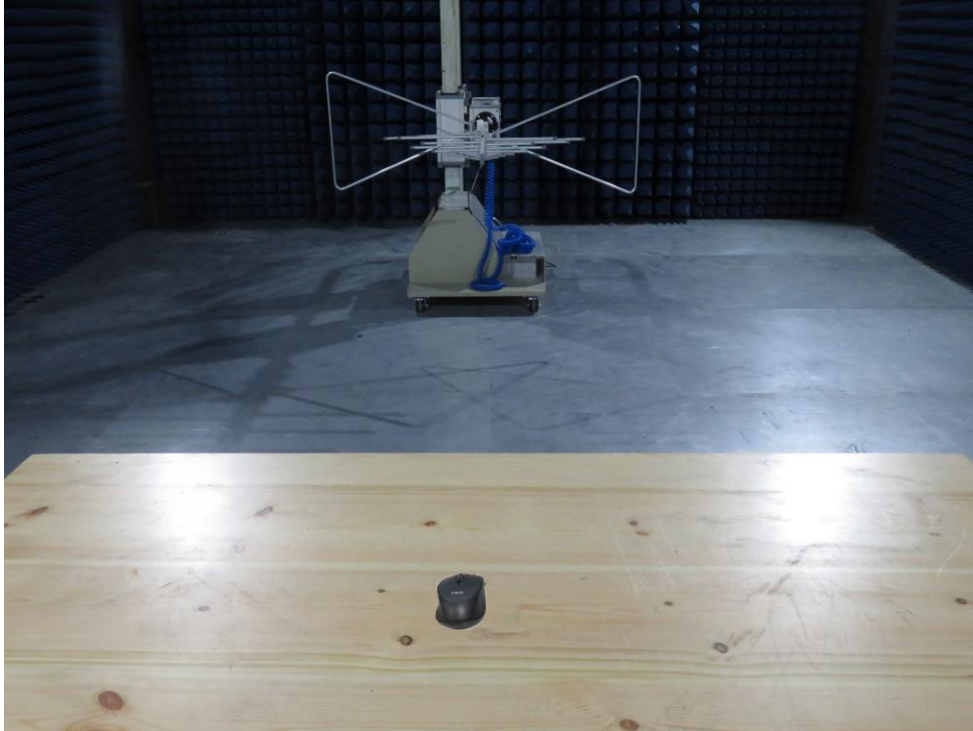
Photo of Radiation Emission Test
