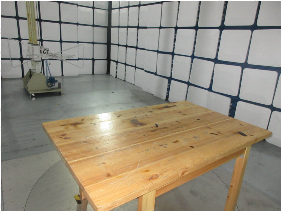
Photo of Radiation Emission Test
