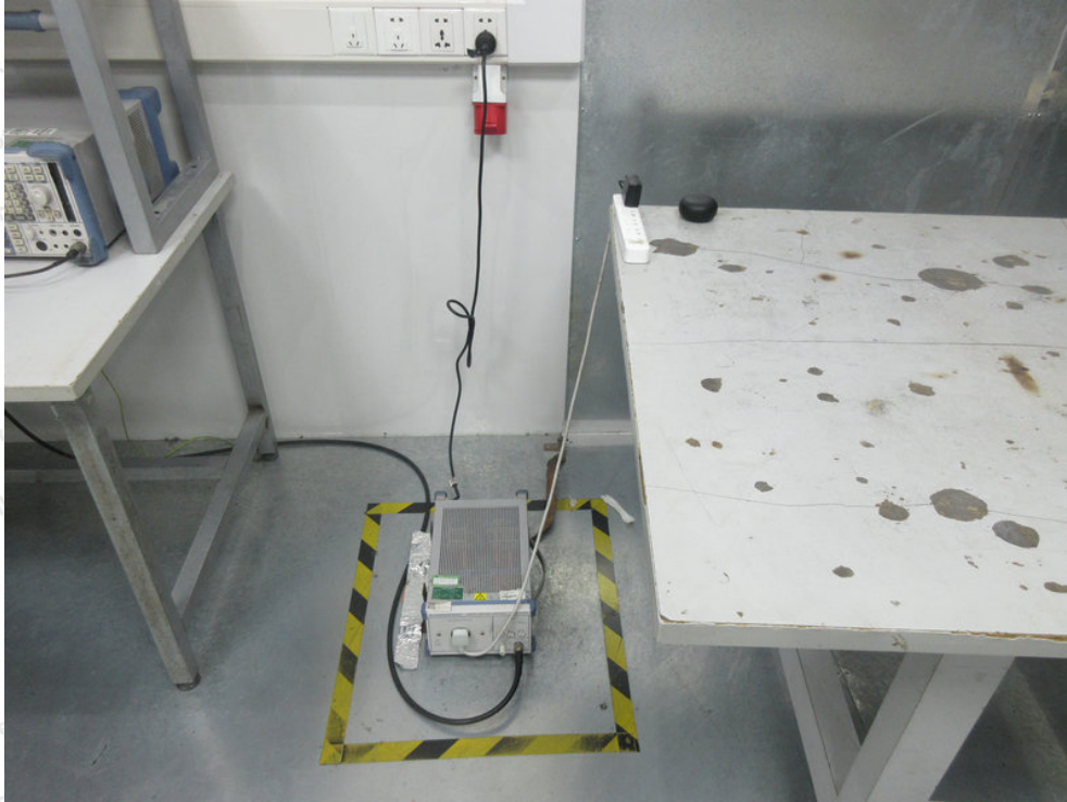
Photo of Conducted Emission Measurement
