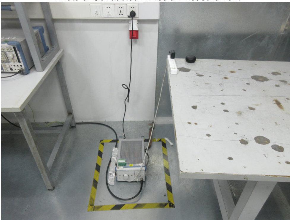
FCC ID: 2A16I-HAKIIFIT Photo of Conducted Emission Measurement
