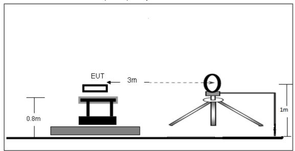
(B) Radiated Emission Test-Up Frequency 30MHz~1GHz
