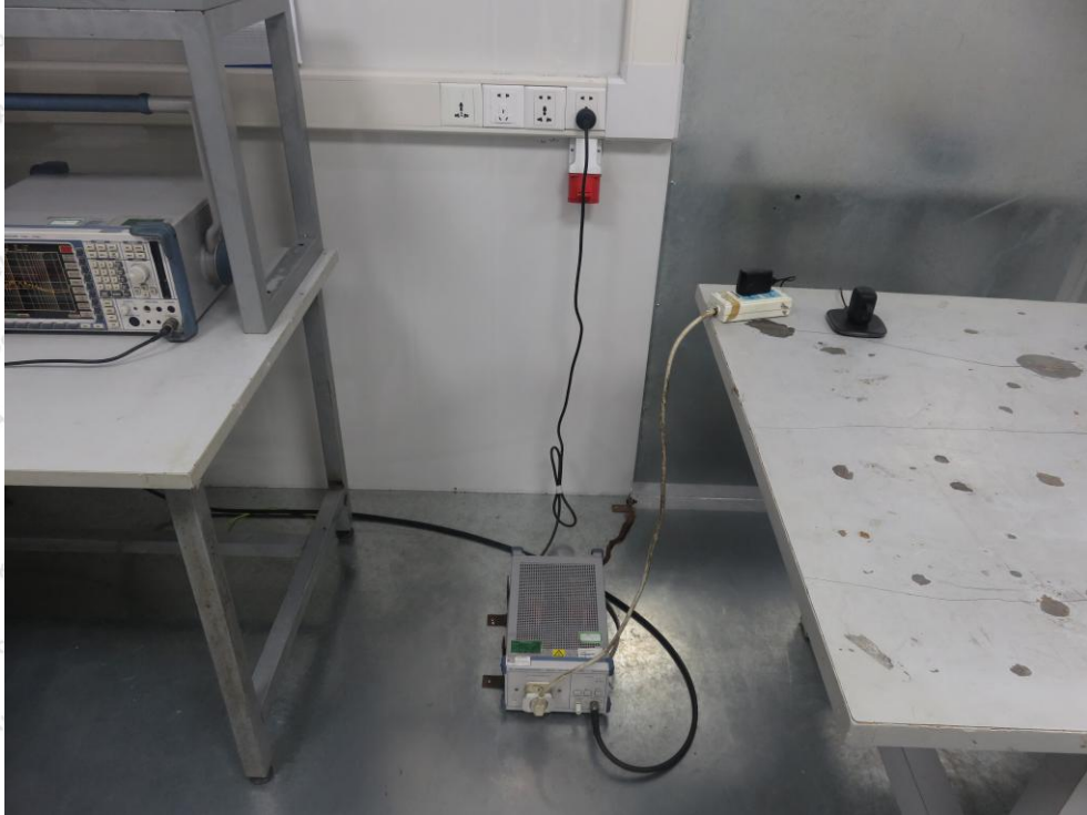
Photo of Conducted Emission Measurement
