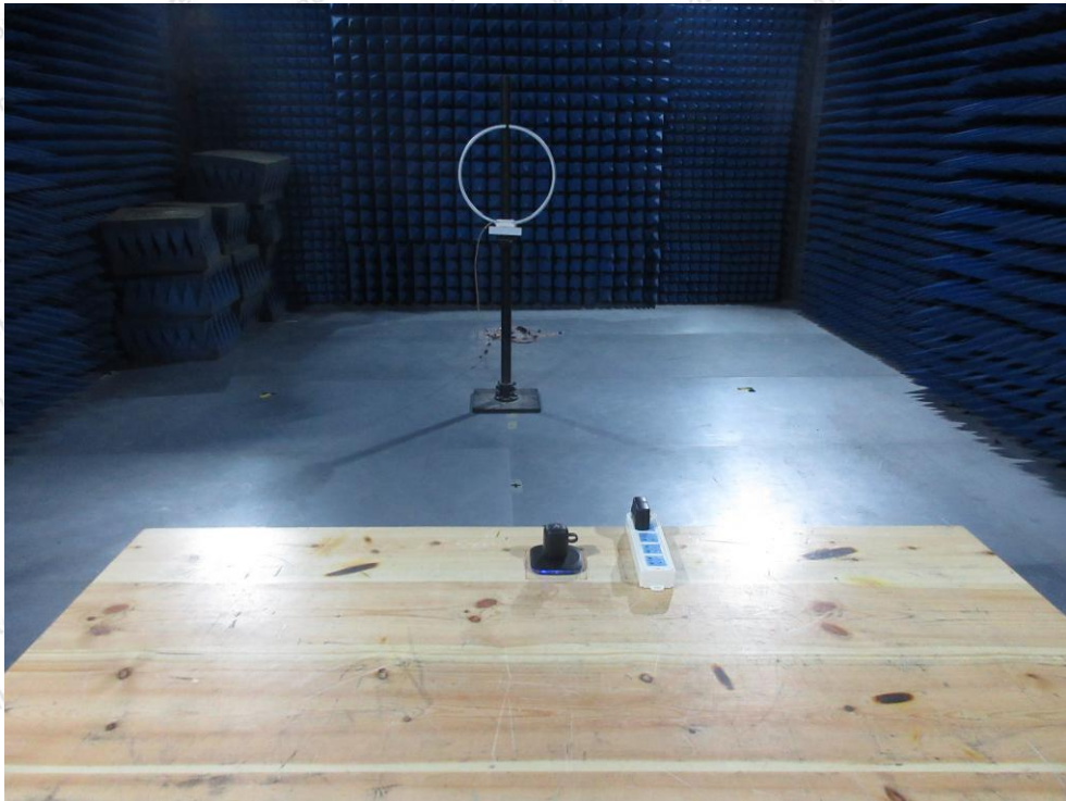
Photo of Radiation Emission Test
