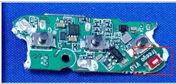
The antenna is Chip antenna.
