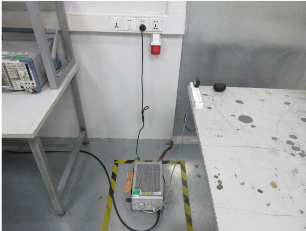
FCC ID: 2A16I-ACTION Photo of Power Line Conducted Emission Test
