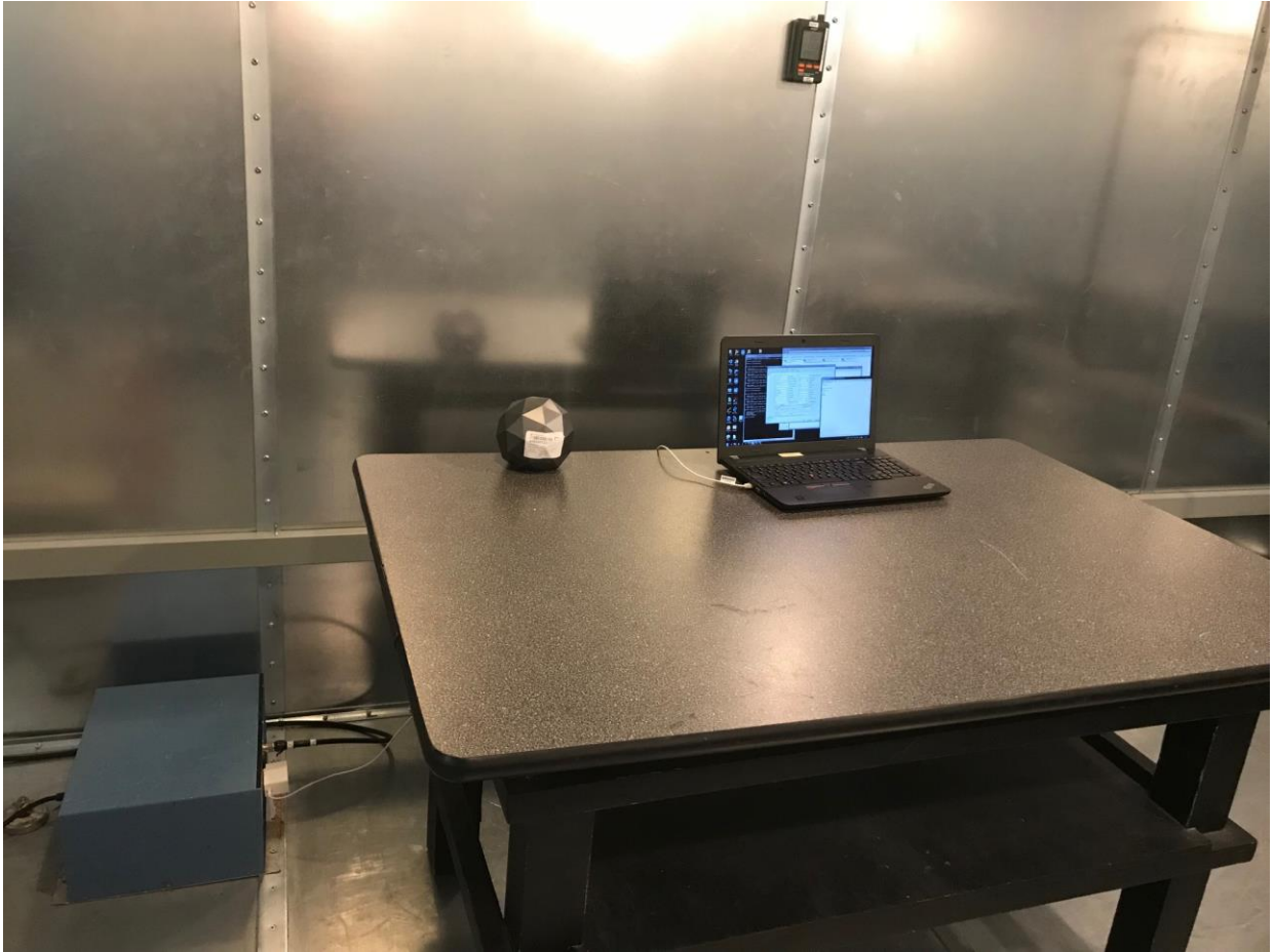
Figure 9: Test Setup for Conducted Emissions - Front (AC Mains)
