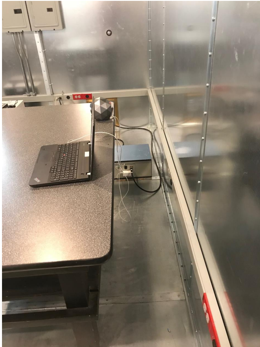
Figure 10: Test Setup for Conducted Emissions - Back (AC Mains)
