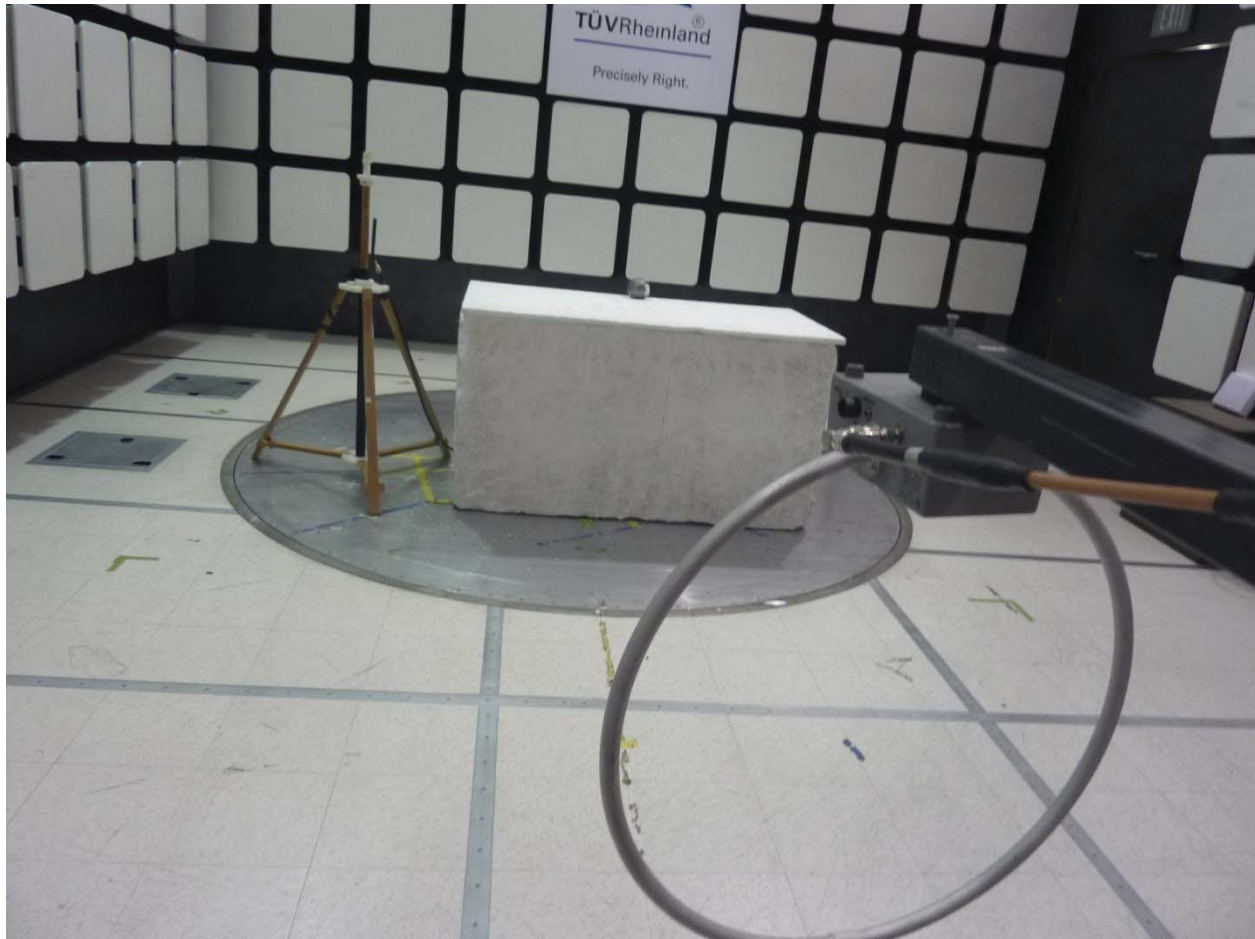
Radiated Emissions 9k-30 MHz front
