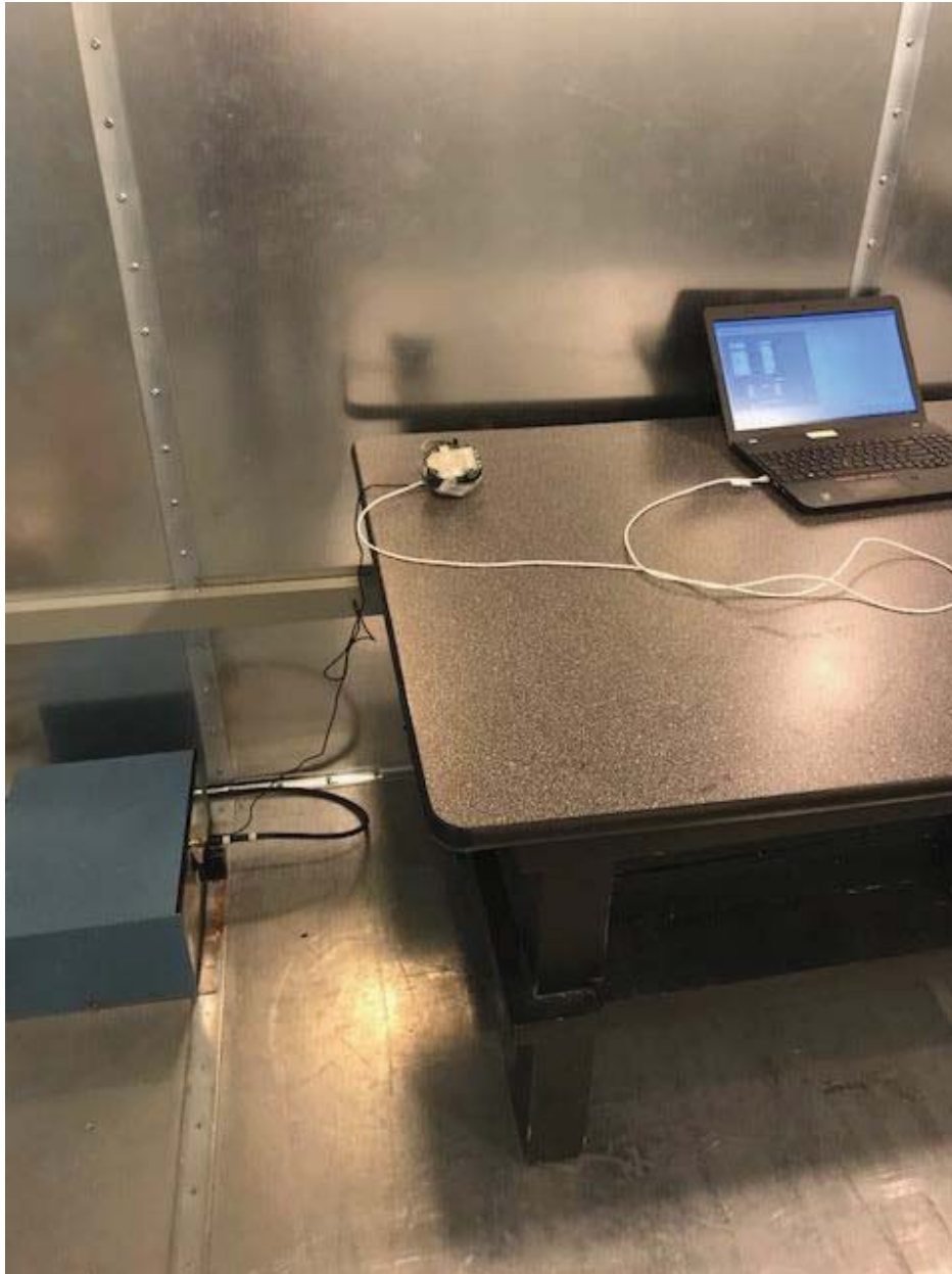
Powerline conducted emissions setup
