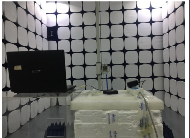
Radiated Spurious Emissions Test Setup Above 1GHz
