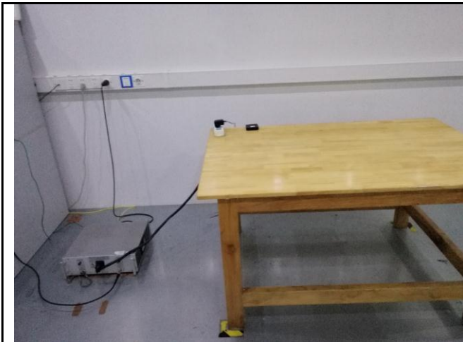
Conducted Emissions Test Setup Front View
