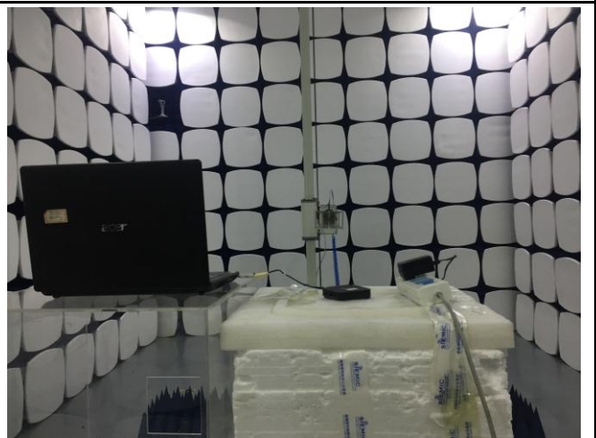
Radiated Spurious Emissions Test Setup Above 1GHz
