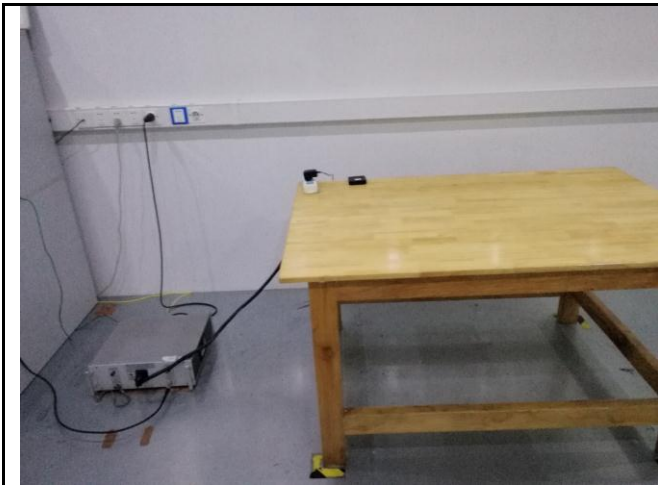
Conducted Emissions Test Setup Front View
