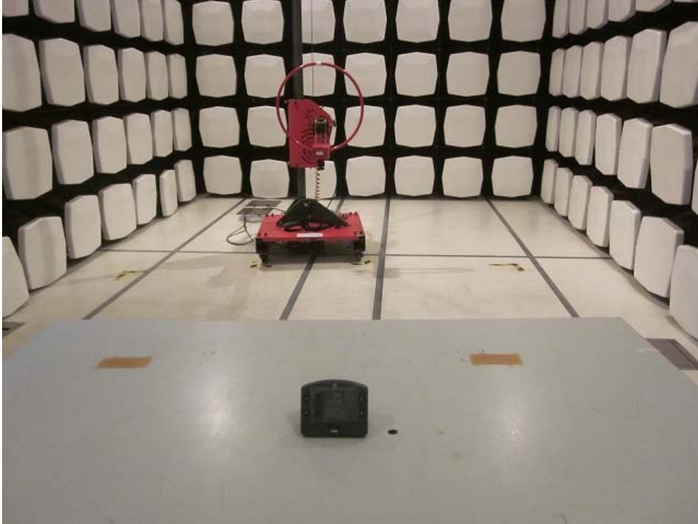
Measurement of Radiated Emission Test Set Up
