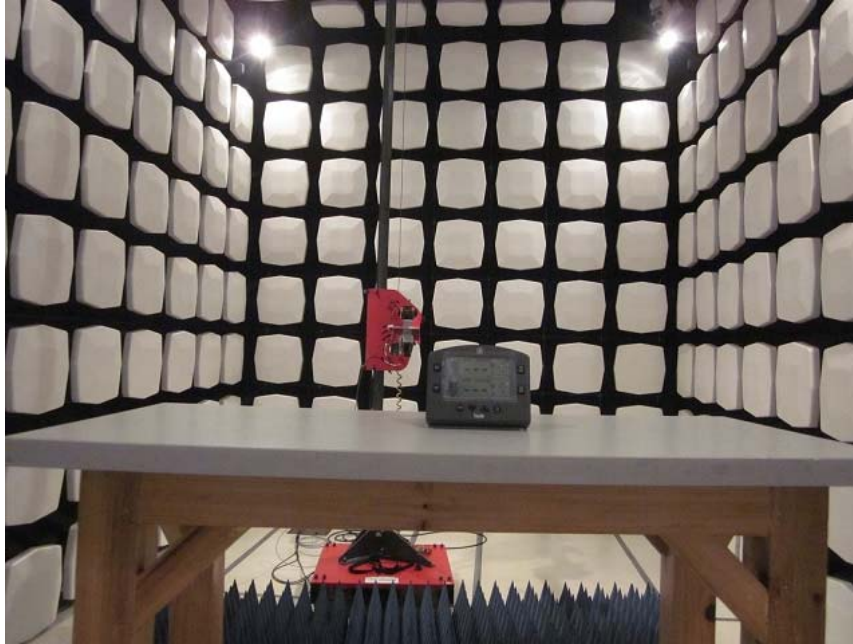
Measurement of Radiated Emission Test Set Up
