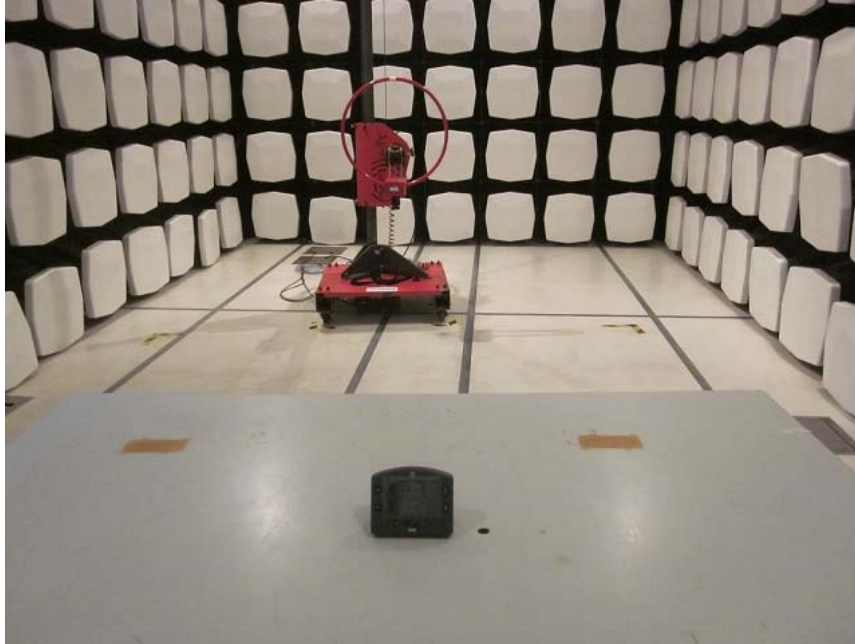
Measurement of Radiated Emission Test Set Up
