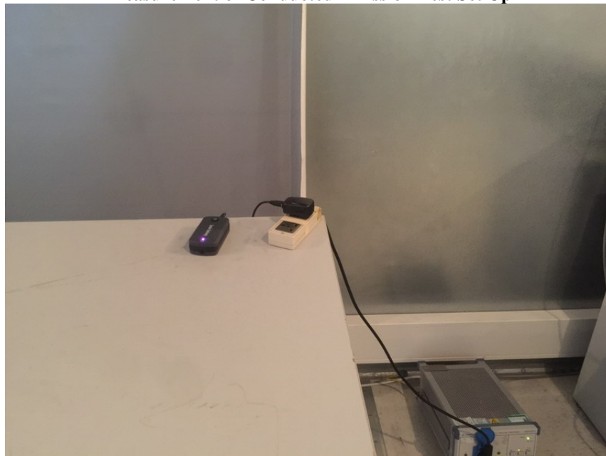
Measurement of Conducted Emission Test Set Up
