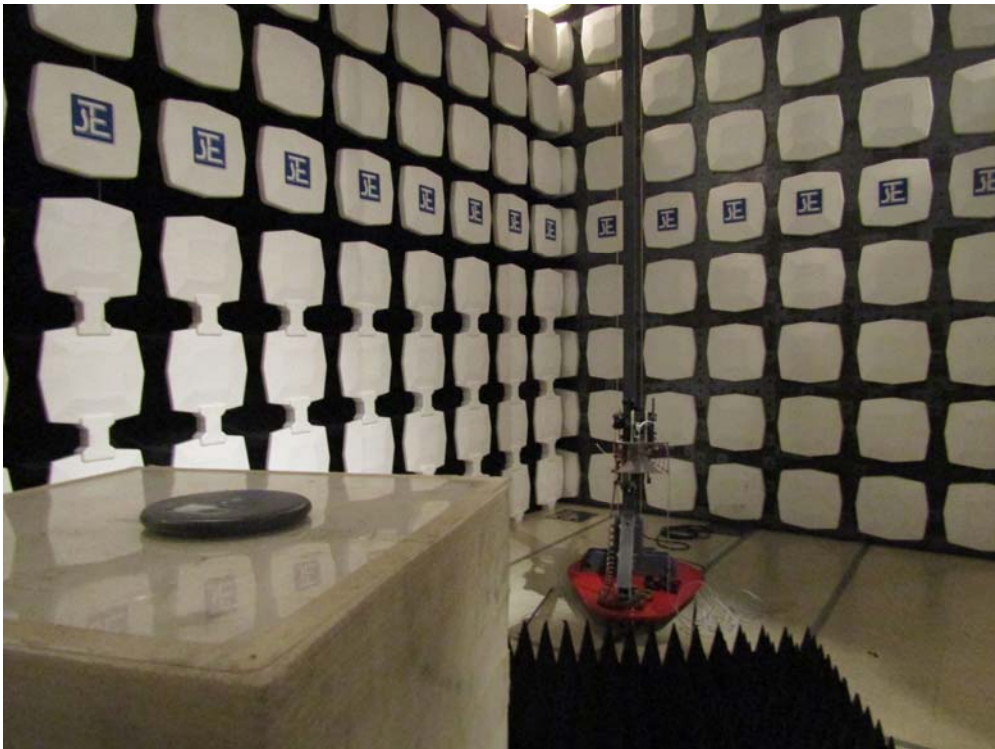
Measurement of Radiated Emission Test Set Up
