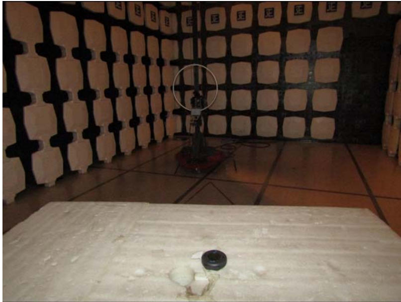
Measurement of Radiated Emission Test Set Up
