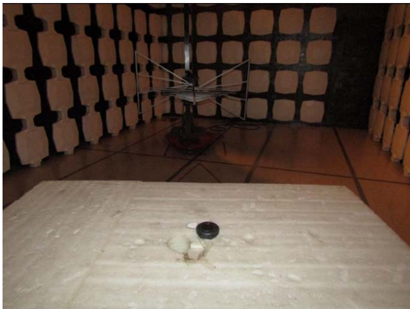
Measurement of Radiated Emission Test Set Up
