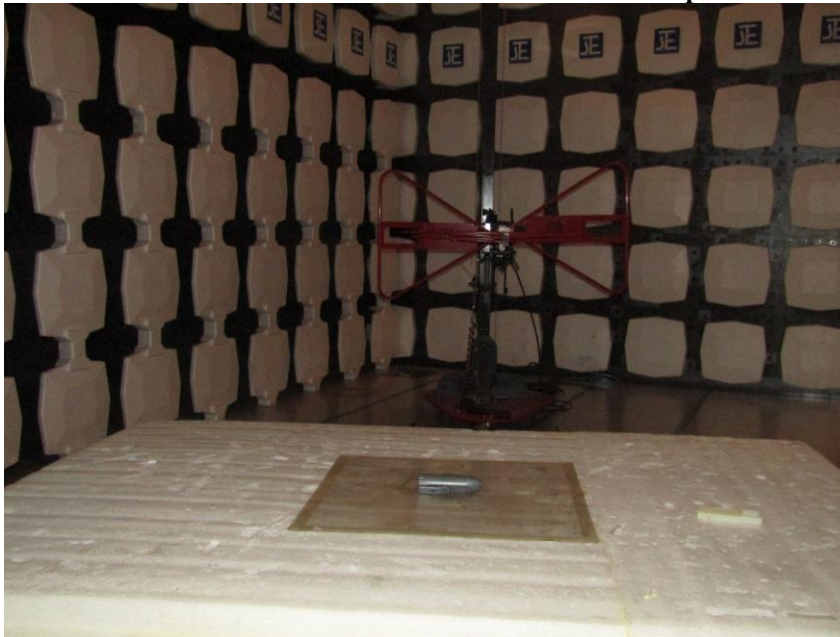
Measurement of Radiated Emission Test Set Up
