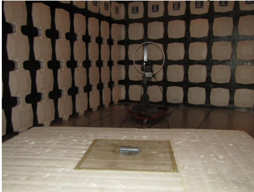
Measurement of Radiated Emission Test Set Up
