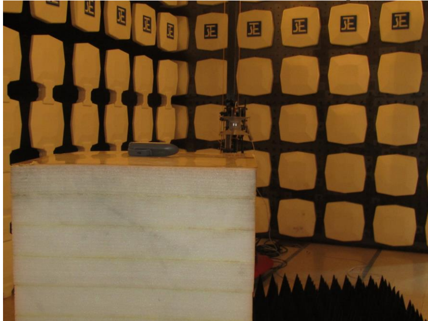
Measurement of Radiated Emission Test Set Up
