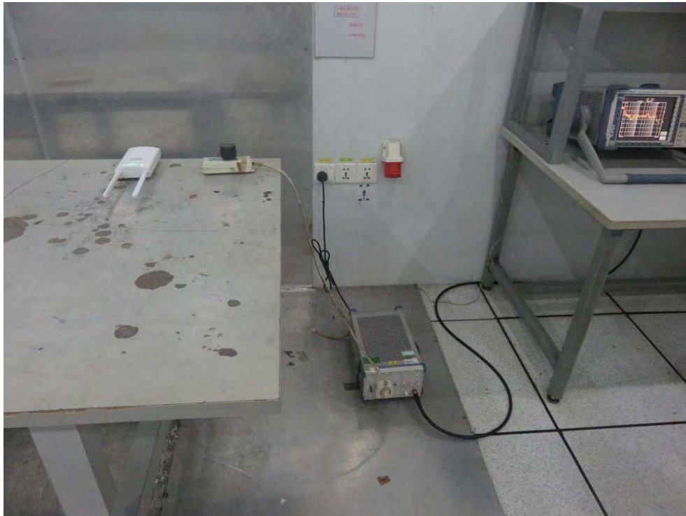
Photo of Conducted Emission Measurement
