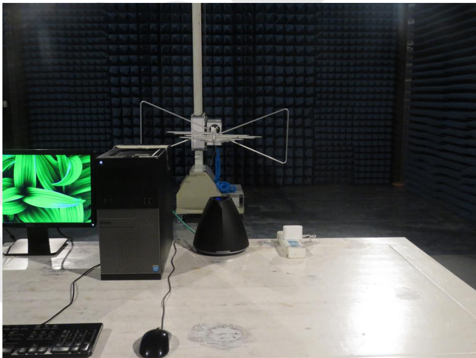
Photo of Radiation Emission Test
