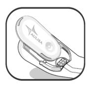
Step 2: Secure the Thermometer Box onto the holder of the Sensor Patch.
