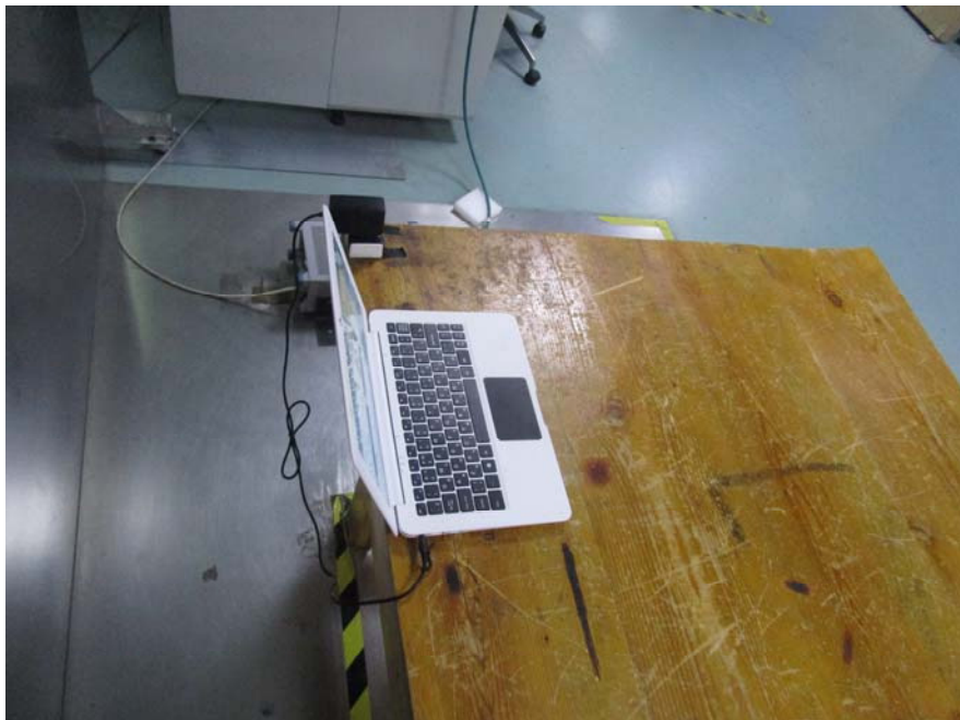
Conducted Emissions - Side View (Adapter #1)
