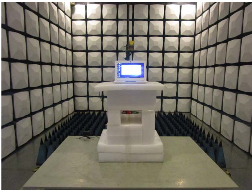
Radiated Emission View (Above 1GHz) (Adapter #1)
