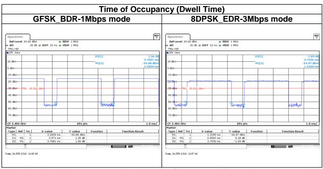
Note: We selected worst case to performed test in middle channel, The results can be meet other channel.
