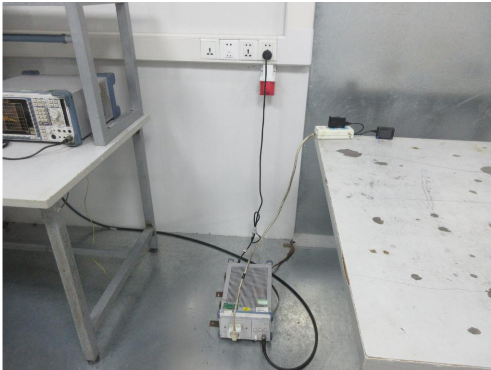
FCC ID: 2A15B-SO64 Photo of Conducted Emission Measurement
