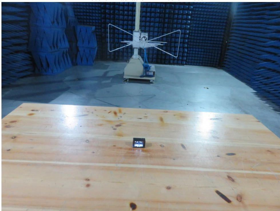
Photo of Radiation Emission Test
