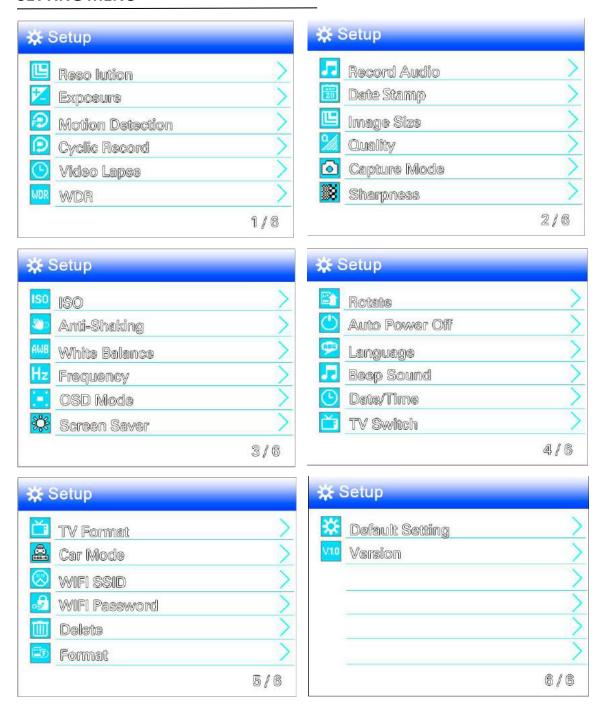
Press the **Power/Mode button** to enter the settings menu, Repeatedly press the **down/on button** to cycle through options and press the **OK button** to select desired option.
