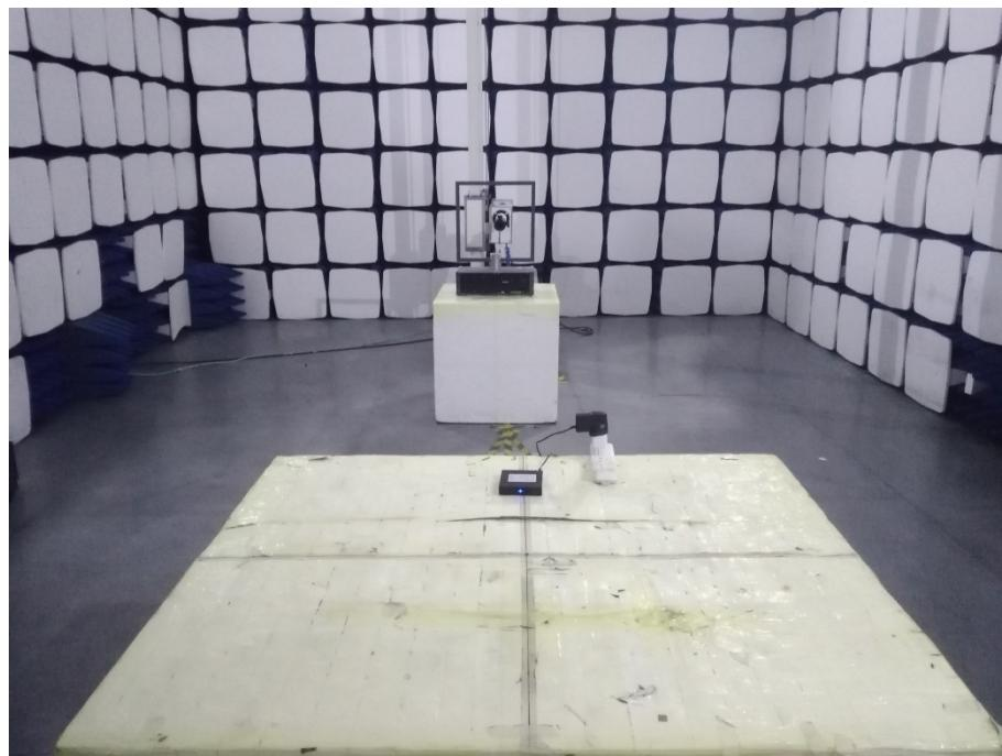
**Radiation Emission Test Setup (30MHz to 1GHz)**
