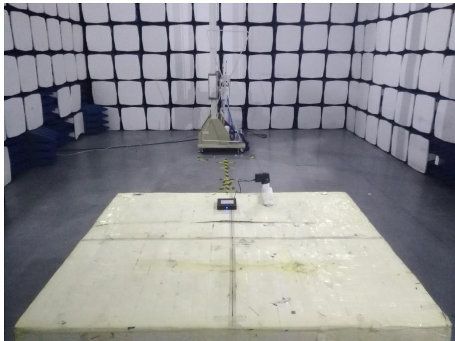
**Radiation Emission Test Setup (1GHz to 18GHz)**
