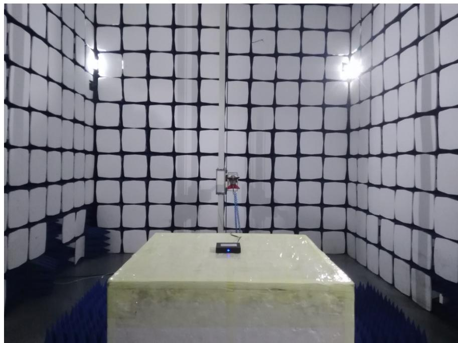
**Radiation Emission Test Setup (Above 18GHz)**
