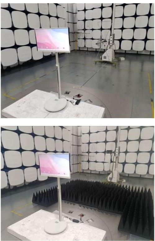
1.1. Photo of Radiated Emission test
