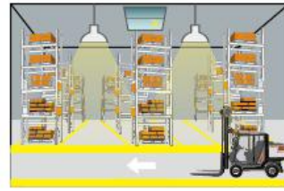
3 After hold time, the lamp gradually dims to a low light level 10% if no movement detected.
