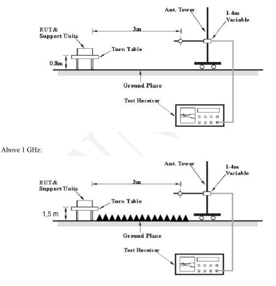
The radiated emission and out of band emission tests were performed in the 3 meters chamber test site, using the setup accordance with the ANSI C63.10-2013 The specification used was the FCC 15.209/15.205 and FCC 15.249 limits.
