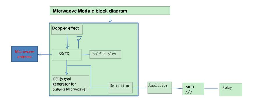
OSC emits a signal at a high frequency 5.8GHz and receives its echo, if a movement in the detection zone changes the echo, the echo signal will be amplified and sent to MCU. MCU processes the signal as high-low-level to control relay.
