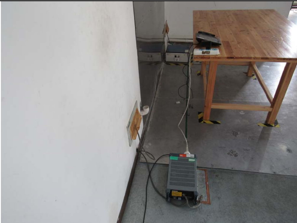
Conducted Emissions Test Setup Side View
