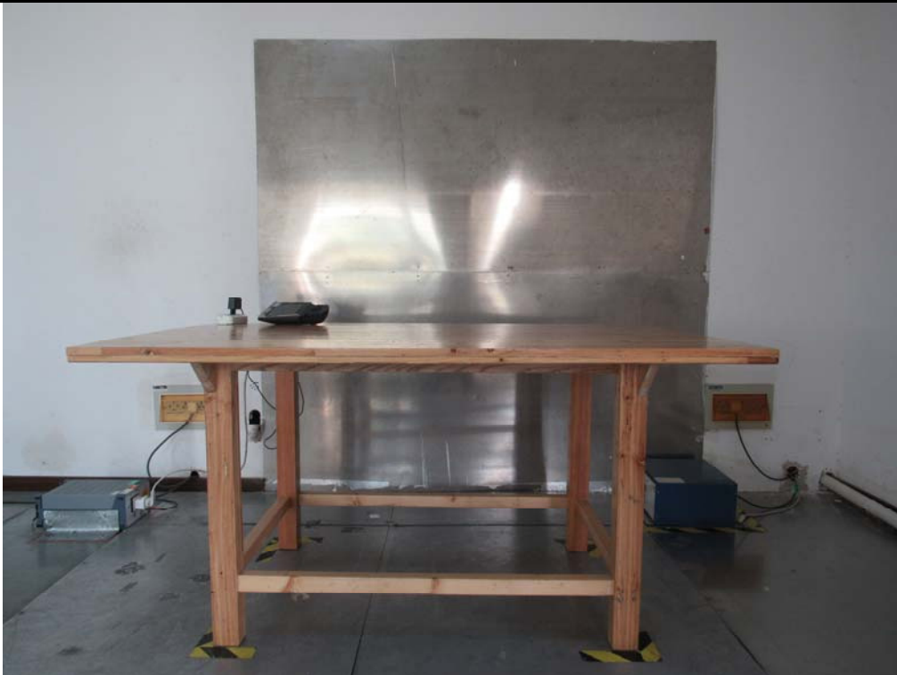
Conducted Emissions Test Setup Front View
