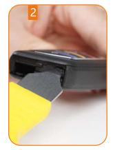
Use the tool into the gap to separate the shell
