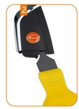
Use the tool into the gap to separate the shell
