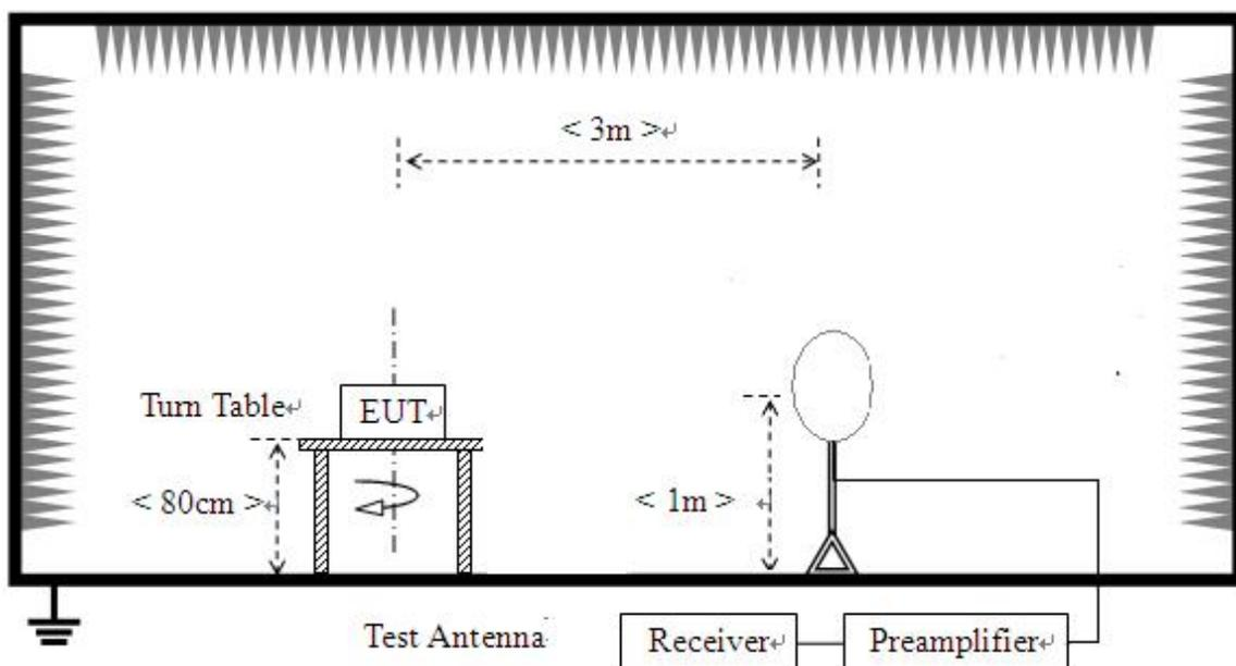
**For radiated emissions from 30 MHz to 1 GHz:**
