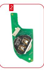
Take the battery out and replace new one Note: The battery type is 2032 with 3V, ensure the positive and negative of battery is correct.
