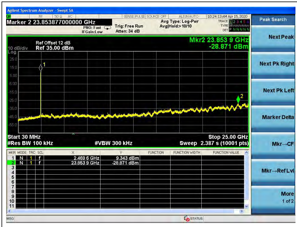
(30MHz to 25GHz, Channel 12, 802.11b)
