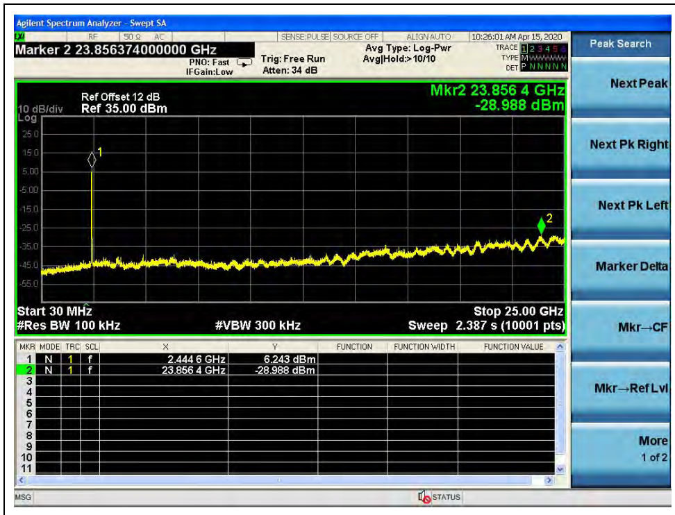
(30MHz to 25GHz, Channel 7, 802.11g)
