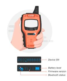
[Start]: press and hold the power button for 1 second [Transponder detection]: press the power button for 1 second [Shut down]: press and hold the power button for 4 seconds [Frequency test]: press and hold the power button for 2 seconds
