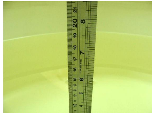
Fig 7.2 Photo of Liquid Height for Body SAR
