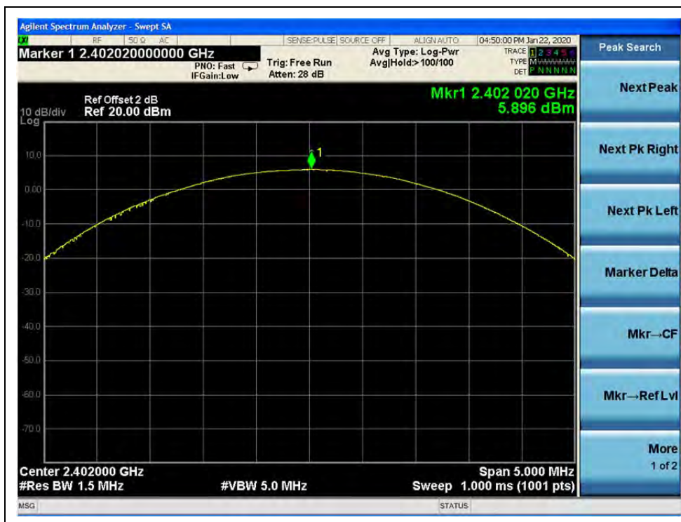
(8-DPSK, Channel 0, 2402MHz)
