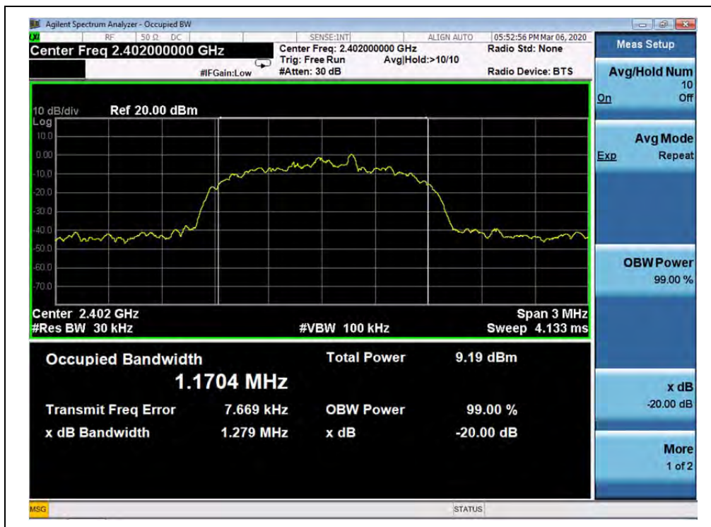
(8-DPSK, Channel 0, 2402MHz)
