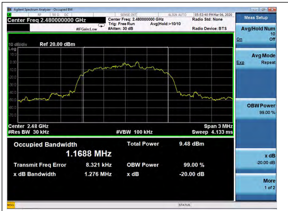
(8-DPSK, Channel 78, 2480MHz)
