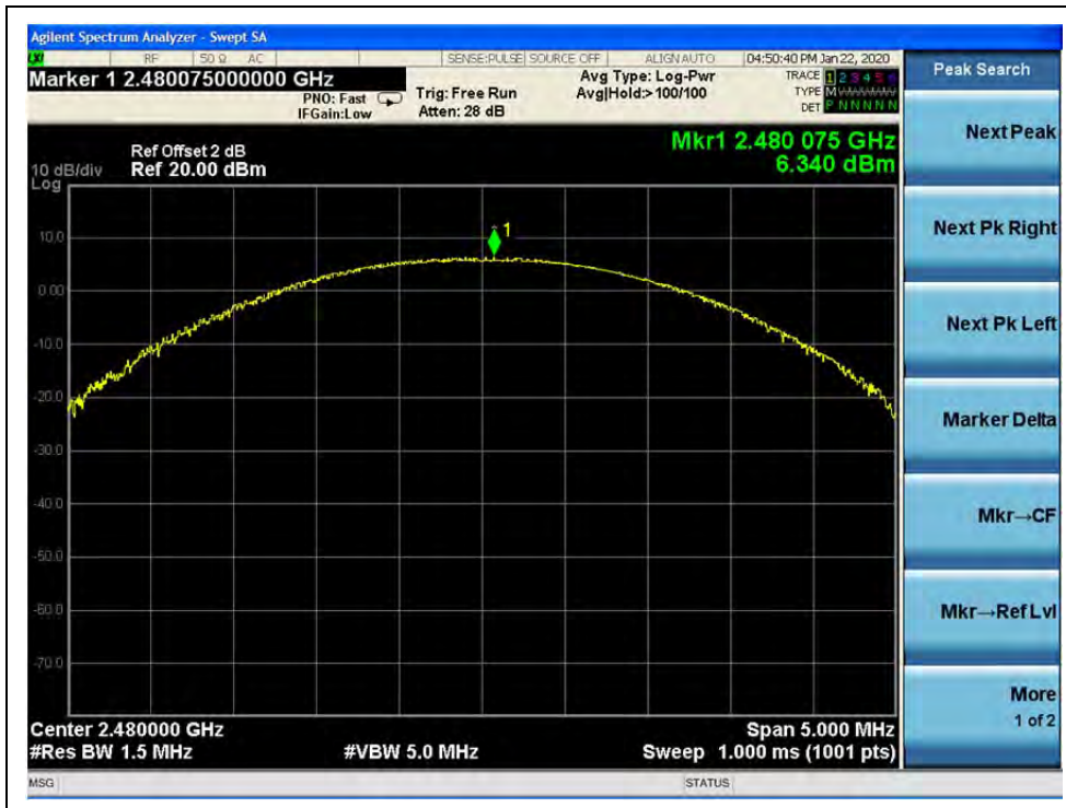
(8-DPSK, Channel 78, 2480MHz)
