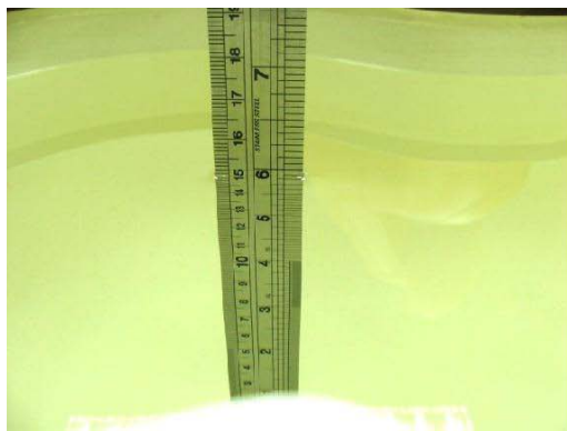
Fig 7.1 Photo of Liquid Height for Head SAR
