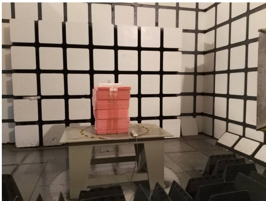
Radiated Emissions View (Above 1 GHz)
