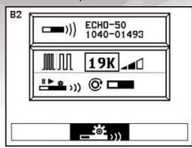
2. Tap to enter Transmitter settings Page. The receiver and Echo transmitter will automatically pair. Then tapor and to select frequency and power level. Tap to highlight wake Up Mode and tap to enter. Then tap or to select desired mode as described below.
