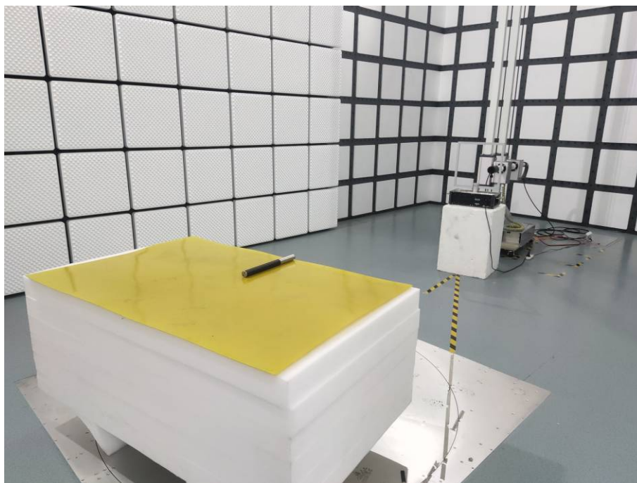
Photo of Radiated Emission Measurement (9kHz-30MHz)
