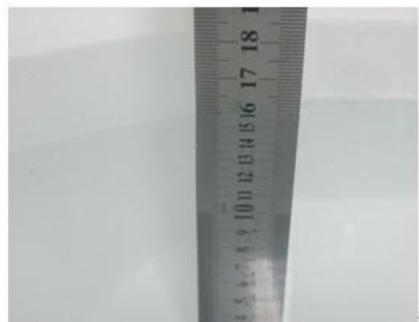
Liquid Height for Body SAR
