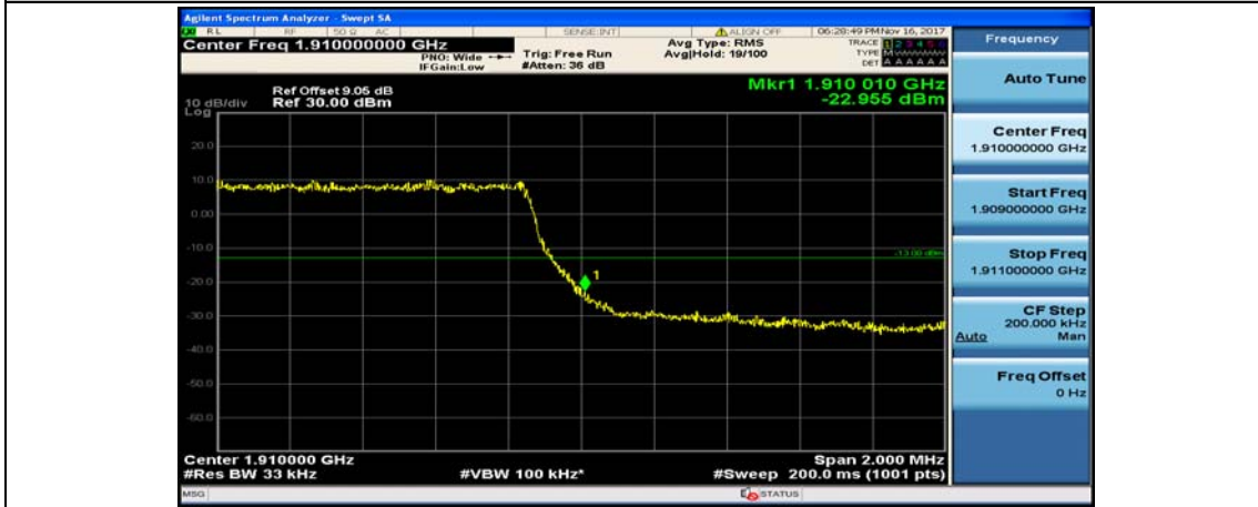
(Channel Bandwidth: 3 MHz)_HCH_QPSK_15RB#0
