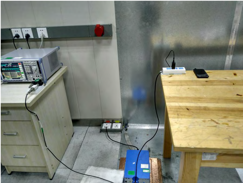
RADIATED EMISSION TEST SETUP
